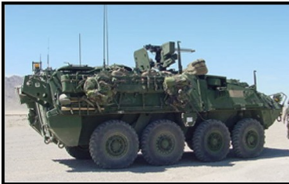
This is a Stryker Infantry Armored Vehicle. Note the wheels. The Stryker is 51% LARGER in exterior footprint than the MTVL, yet offers no more interior volume.
