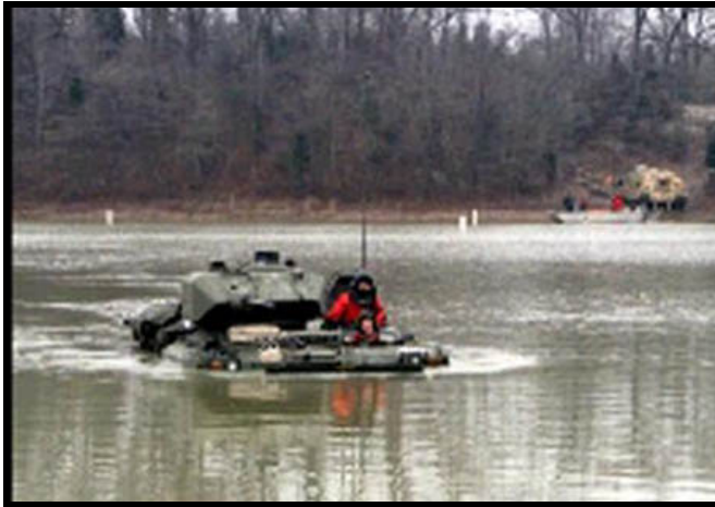
This shows an M113 (equipped with a turret) swimming using its tracks for propulsion. The Stryker cannot swim.
