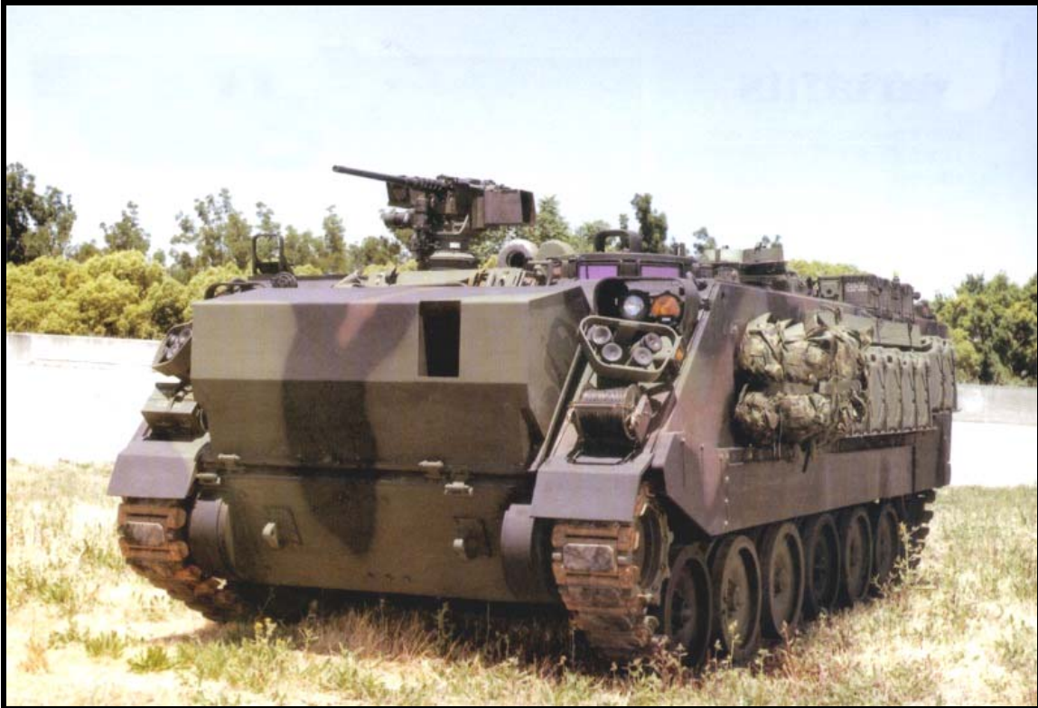
This is the remarkable MTVL, a major upgrade and stretched version of the M113A3. Note the 6 wheels.
