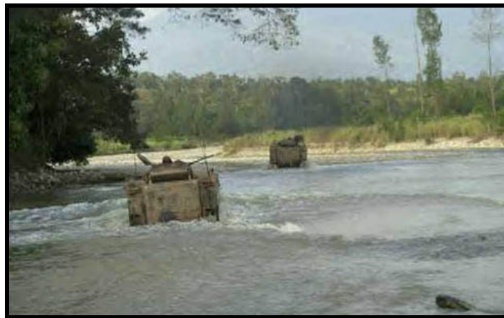
The Australians tried wheeled armored in east Timor without success. They switched to tracked M113s which worked fine, both on and off road.
