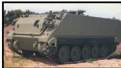
This is the tried and true M113A3 (only 5 wheels), the precursor of the MTVL.
