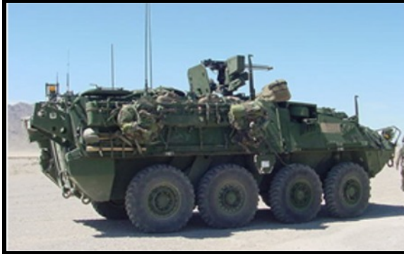
Stryker. Note wheels and sheer size of the vulnerable near shoulder height wheel area. Poor off road and urban performance. Impossible to up-armor properly against RPGs.
