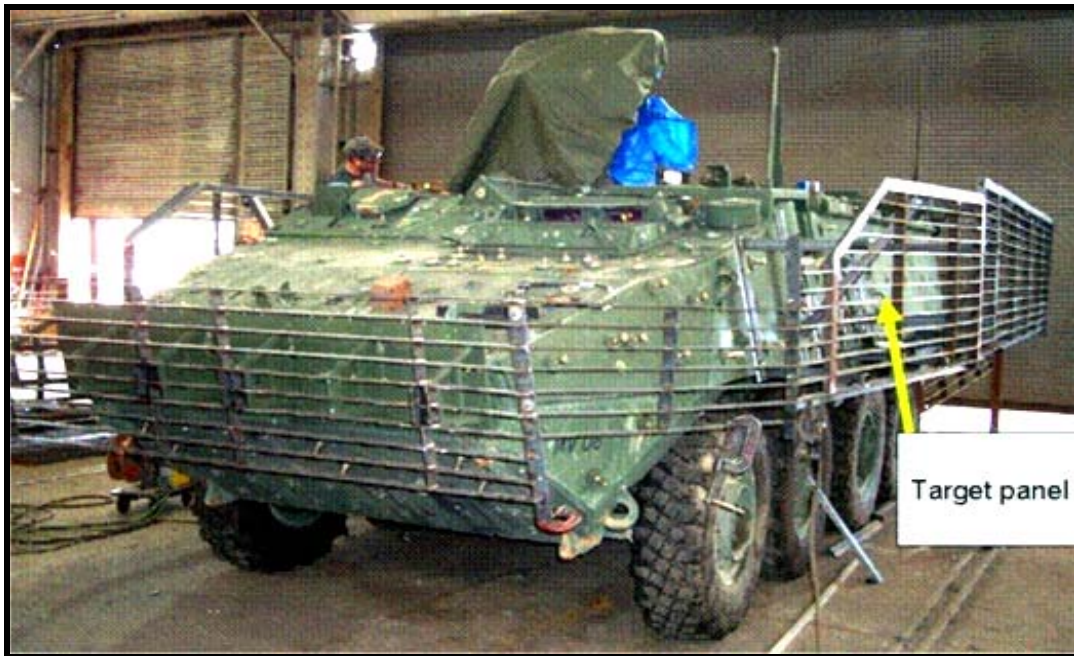
August 2003 picture of a Stryker being fitted with a decidedly primitive Anti-RPG shield. Note that top and the wheel well area remain entirely vulnerable.
