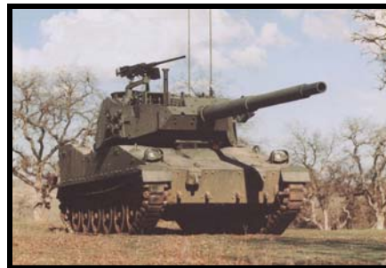
This is the M8 AGS Armored Gun System. Note the tracks. It is US Army Type Classified.
