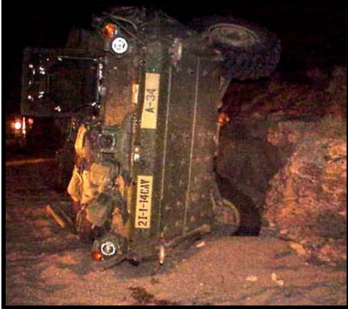
The center of gravity of the Stryker is too high. It is NOT stable and overturns.
