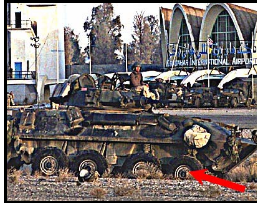
Marine LAV 25 in Afghanistan. Note the severely damaged tires.
