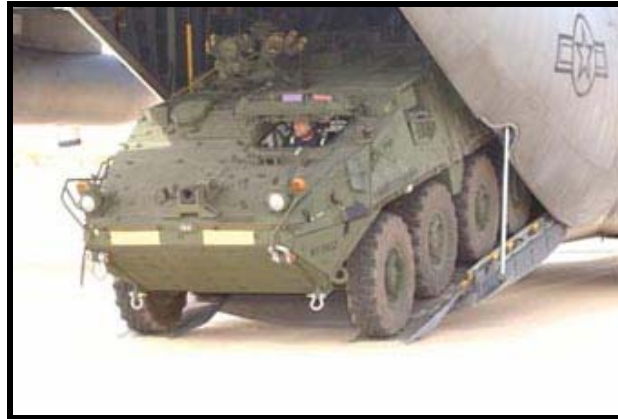
Stryker just squeezes into a C-130 but is too heavy to fly any useful distance. Some variants are too heavy for C-130 to take off!
