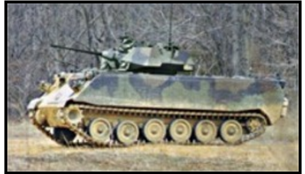
MTVL. Note tracks. Excellent off road and urban performance. Tracks plus inherent design means can be up- armored against RPGs. Turret is optional
