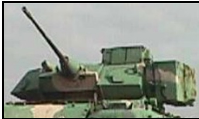
Bradley 25mm chain gun outranges small arms and RPGs and significantly enhances offensive capability and survivability
