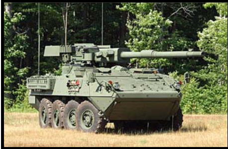
This is a Stryker Mobile Gun System. Note the wheels. It has terrible off road performance & overall just does not work.
