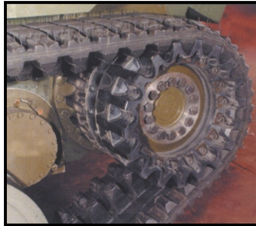
Band Track, a continuous band of rubber composite with a steel core, gives a smoother, quieter ride, allows faster top speeds, and is lighter.
